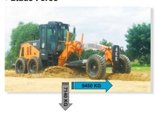
Best in class Drawbar Pull Force of 9450 Kg for high productivity. Blade Down force of 7140 Kg for faster cutting and effective grading operations.
