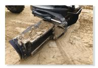
Hydraulically operated adjustment of blade tilt angle from the cabin. Ensures no stoppage of work for blade adjustment.
