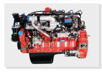
Ashok Leyland H-series 6 cylinder water cooled Turbocharged Diesel engine with SCR technology generating 180 hp @ 2200 rpm meeting CEV Stage-IV emission compliance. Common Rail Fuel System for effective power strokes and efficient fuel consumption. This high torque engine provides high pushing power and thus improves operating efficiency.
