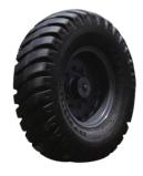
Heavy duty rock grade tyres of size 14.00 X 25 with 20 Ply rating for minimum wear and increased life.
