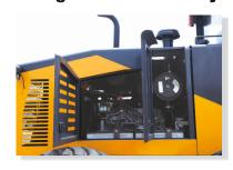
Open vents from either side ensures easy access from ground level for daily maintenance checks, serviceability and adequate ventilation.
