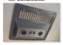
Roof mounted AC is provided to ensure operator comfort and efficiency.
