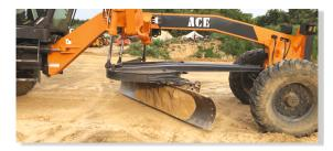
360° rotation of the blade also ensures productivity during reverse movement of the grader, specially in heap breaking application. Offers high productivity in minimum no. of passes saving fuel, time and maintenance cost.
